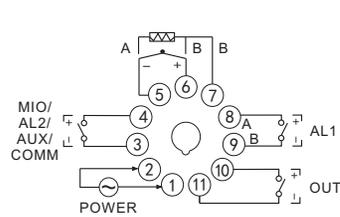
Note: 4~20mA input can be externally connected to 25Ω resistor to become 100~500mV voltage signal, then input from 5th and 6th terminals.
