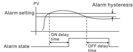
The power-on alarm ON delay also takes effect. When the alarm ON interval is below the ON delay setting, the alarm output will not turn ON. Similarly, when the alarm OFF interval is below the OFF delay setting, the alarm output will not be turned OFF.
