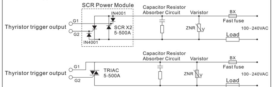
Note 1: According to the voltage and current of load, choose suitable varistor to protect the thyristor. Capacitor resistor absorber is needed for inductance load or phase-shift trigger output.
